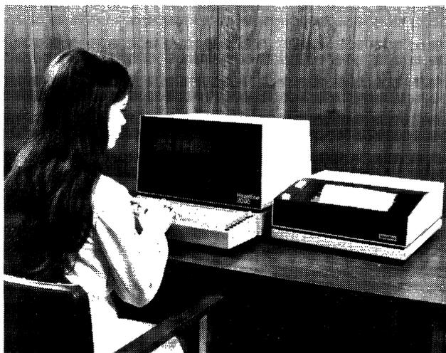
*The Hazeltine 2000 is the most popular display terminal of the five models offered by the company. Included with the terminal shown above is the optional 30 cps thermal printer. The Hazeltine 2000 is marketed as a direct replacement for Teletype Model 33 and 35 units.*
