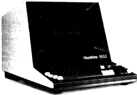
A DEC VT-52-compatible Hazeltine terminal providing the user with additional key functions not available with the VT-52, programmable key switch, audio feedback, field tab, and line insertion/deletion features.
