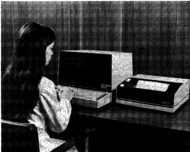
The Hazeltine 2000 is the most popular display terminal of the six models offered by the company. Included with the terminal shown above is the optional 30 cps thermal printer. The Hazeltine 2000 is marketed as a direct replacement for Teletype Model 33 and 35 units.
