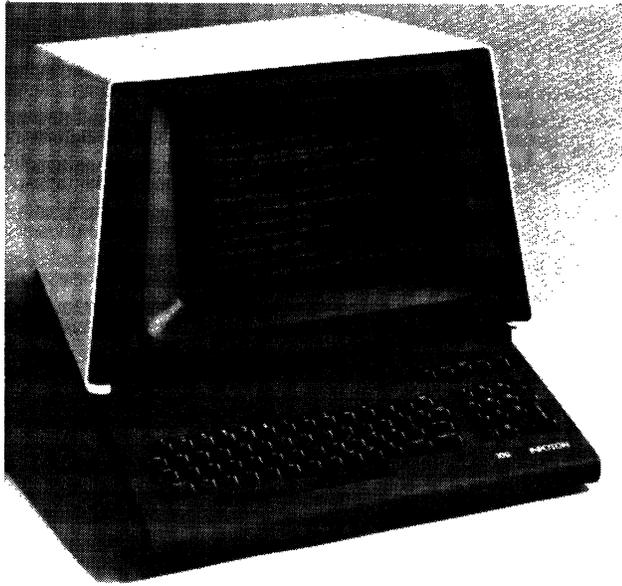
The Infoton 100 shown above is a low-cost, microprocessor-based display terminal offering screen formatting and editing, paging, and line drawing features.
