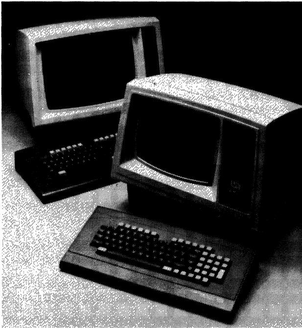
*The ADM 32 features Lear Siegler's new ergonomic design, including a detachable keyboard and a 12-inch non-glare display screen. Options available include a six-position tilt mechanism, a 15-inch display screen, and green phosphor characters.*
