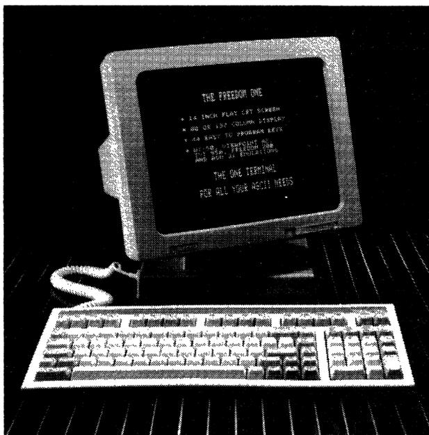
*The Freedom ONE video display terminal provides the customer with low price and advanced features, in one terminal. Being fully compatible with the company's Freedom 200 model, the Freedom ONE's emulation modes include Wyse WY-50, TeleVideo 950, ADDS Viewpoint A2, and Lear Siegler ADM 31. This terminal bridges the gap between low-price, low-featured products and high-priced, full-featured products, giving it universal appeal.*
