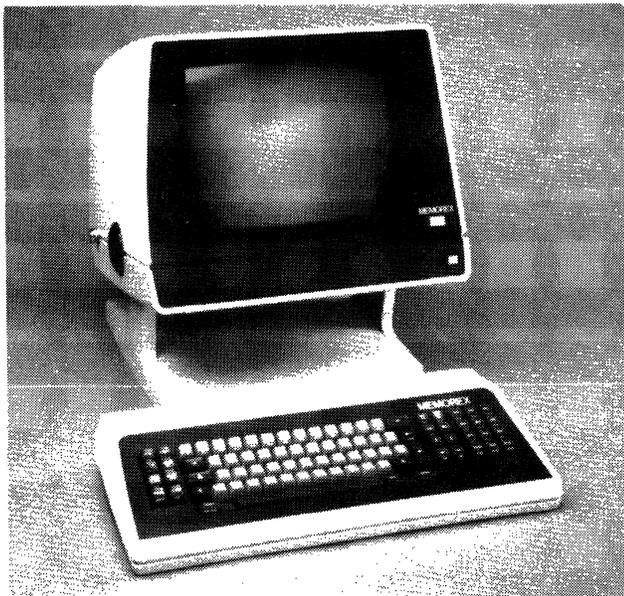
Another new addition to the Memorex product line is the 2080 display station. The 2080 provides four operator-selectable display capacities, ranging from 1,920 to 3,564 characters.
