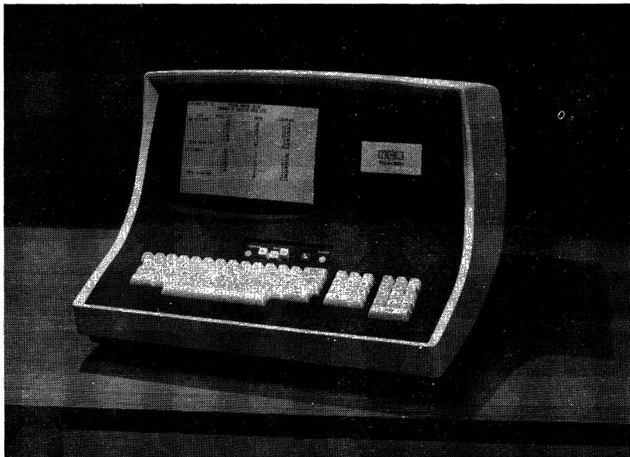
A low-cost family of Teletype-compatible stand-alone CRT keyboard/display terminals.
