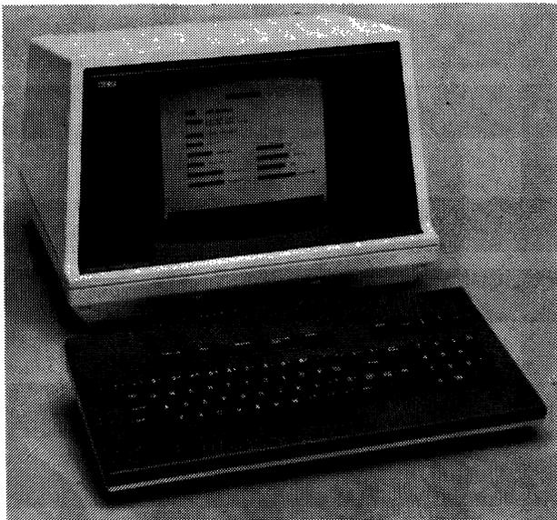
The NCR 7900 terminals are available with a detachable keyboard option. The Model 1 (shown here) features interactive operation enhanced by a number of video attributes.
