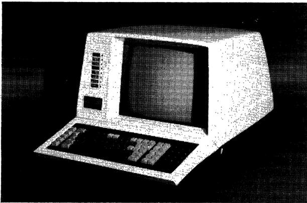
A PTS 100 system can include from 1 to 32 CRT display units, as well as a variety of auxiliary I/O devices. Display screen capacities of 480, 960, and 1920 characters are available.
