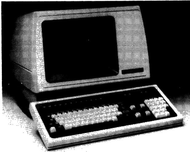
The Model 940 Electronic Video Terminal is intended to be the first member of Texas Instruments' OPTI 900 family of displays. A unique feature of the Model 940 is its ability to divide the display screen into as many as 12 independent scrolling regions.
