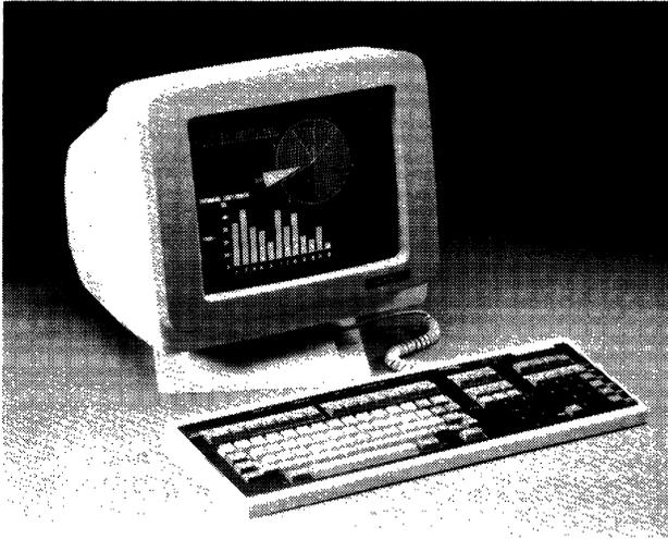
*Teleray's Model 7-7305 is a multiprotocol terminal that features complete software- and keyboard-compatibility with the Honeywell VIP7305, as well as a keyboard-selectable DEC VT102 mode. The Model 7-7305 incorporates Teleray's new Triumph enclosure design, and features a keyboard with a layout identical to that found on the Honeywell keyboard.*
