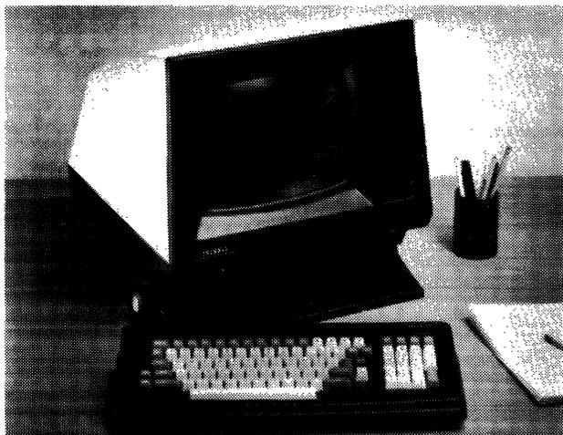
*The Teleray Model 100 is a DEC VT100 emulator. The Model 100 is shown here with a 12-inch display screen and the N-style enclosure. All Teleray terminals can be configured with a 15-inch screen as well as the 12-inch size; in addition, six other enclosure styles are currently available.*
