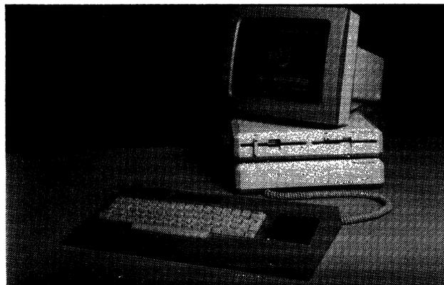
▶ The Telex 1186 Intelligent Workstation may be configured as part of a 3270 network via a coax interface board. The MS-DOS operating system is supported for IBM Personal Computer compatibility.
