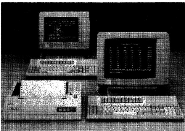
*Two terminals in the Telex System/3X product line are the 079-2, 12-inch color terminal, which displays characters in seven colors, and the 180-2, 15-inch monochrome display terminal, which features green or amber phosphor.*
