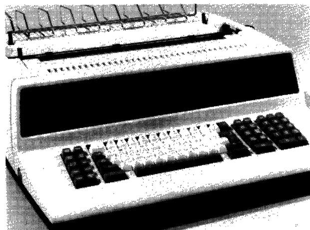
*The Telex 767 Keyboard/Printer Terminal is equipped with a console panel which includes LED indicators, a 3-digit display, and a touch pad. Model 2, pictured here, provides a metalized printwheel mechanism for letter quality printing.*
