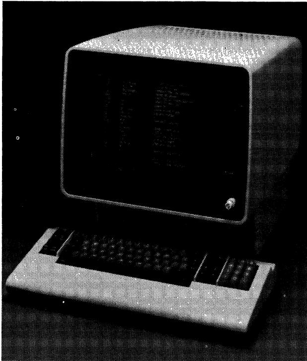
The 310 is Telex's first entry into the ASCII terminal market. Features include a 15-inch display screen, detachable keyboard, and character or block mode transmission.
