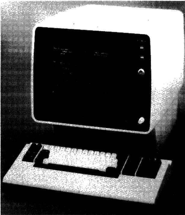
Telex has added SDLC capability to the 276 Control Unit Display Station. The 276 offers control of up to eight devices, and is functionally compatible with the IBM 3276.
