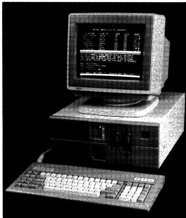
*The Telex Intelligent Workstation with 5250 Emulation Option allows the operator to switch between System/3X host sessions and Intelligent Workstation application programs.*
