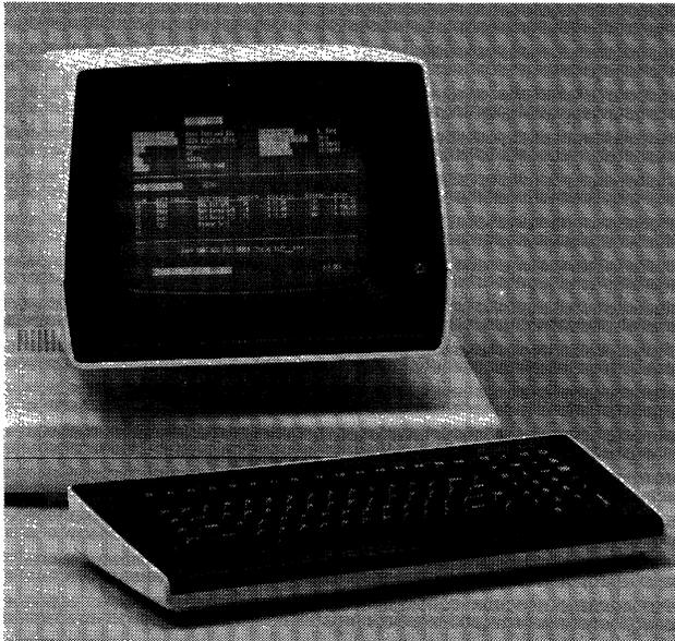
*The Cobra is Zentec's smart video display terminal for OEMs and system integrators. The terminal is modularly designed, consisting of three separate components: the CRT module (available with 12- or 15-inch screen); the logic module; and the keyboard. The display module is mounted on a ball and joint mechanism, enabling the user to tilt or swivel the display for the most comfortable viewing position. The keyboard is detached.*
