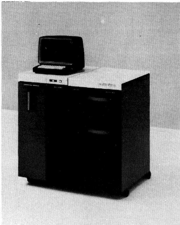
The B 867-1 System and Communications Processor accommodates seven communications lines, and up to 114K bytes of main memory. On the right is a dual cartridge disk drive.
