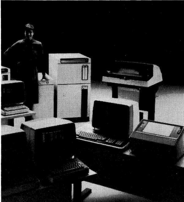
Burrough's latest CP 9500 Series offerings, Models CP 9558 and CP 9572, contain from four to eight independently operating processors that permit the system to be used in a wide variety of transaction-oriented environments. The processor system shown above includes a new Burroughs B 9494 disk drive, B 9246 line printer, and a cluster of Burroughs BMT display terminals.
