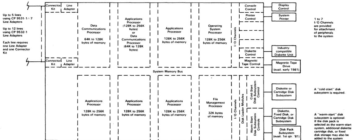
CP 9558 configuration includes one operating system processor, one file management processor, one data communications processor, and two applications processor as standard components. Two additional applications processors, or one applications processor and one data communications processor, may optionally be added, for a total system maximum of six processors, or 1.2MB of aggregate main memory.
