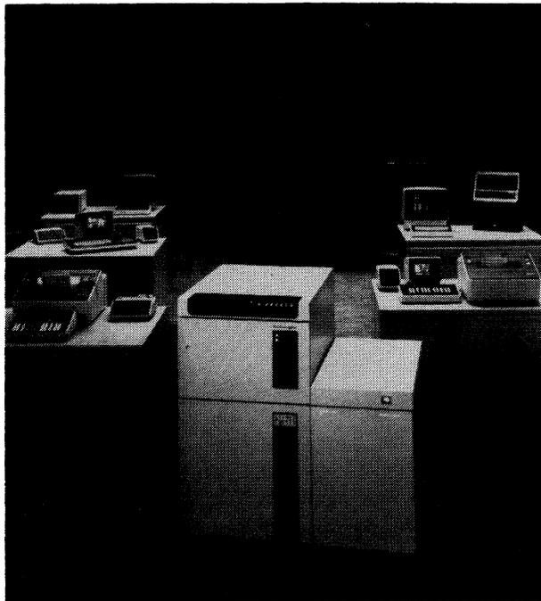
*Burroughs CP 9582 communications processor system (foreground center), shown here with various related Burroughs terminals, serves as a financial controller system, manufacturing data collection system, and general purpose terminal control and distributed processing system. The CP 9582 performs line protocols, message handling, and screen formatting functions for the terminals. It then passes the edited transactions to a Burroughs or non-Burroughs computer for processing.*
