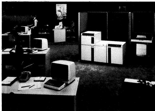
*Burroughs CP9500 system (right of center) is shown here with the B 9350 line expansion module (abutting main cabinet) and a B 9246-6 600 LPM printer.*
