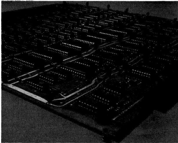
Front end processors come in many sizes. Above is the DCU/50, which is contained on a 15-inch square circuit board, and fits into one I/O slot in a Data General NOVA or ECLIPSE processor.
