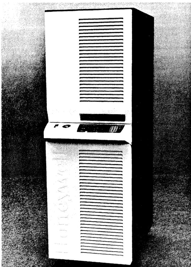
*Honeywell's DATANET 6661 network processor is offered as a front-end for Honeywell mainframes in pre-DSA network environments. It supports large and very large systems that run GCOS, GCOS 8, or Multics operating software.*
