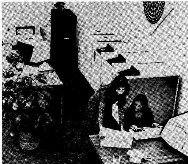
The new components (in design model form) of the IBM 8100 Information System are shown above. The five cabinets on the right contain, starting from the back of the room, two 8809 tape drives, processor (in the middle), and two storage input/output units. The new 8875 display terminal is in the foreground.
