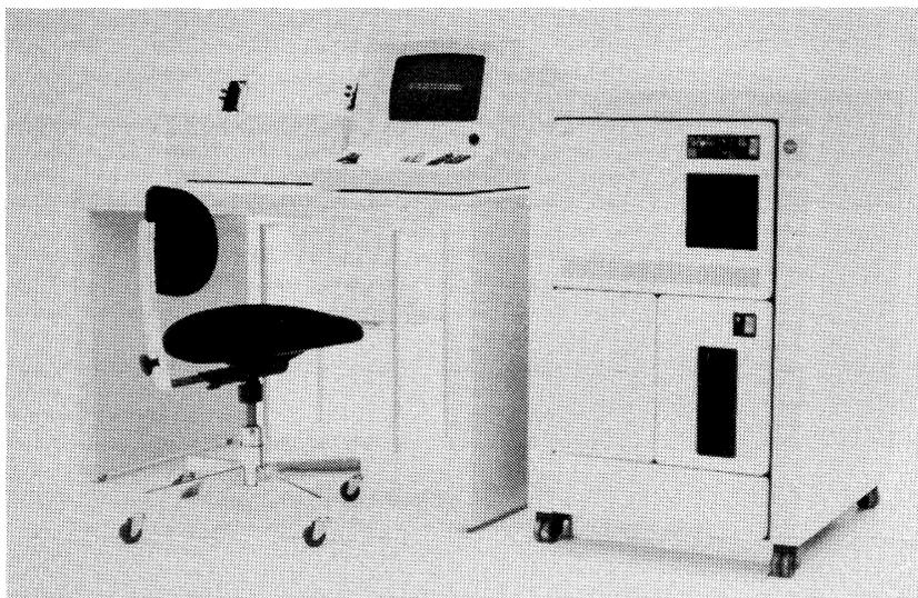
*The Series/1 as shown, includes a low-boy rack enclosure housing the processor and a 4964 diskette unit. The 120-cps 4974 printer is shown at left. The 1,920-character 4979 display station is also shown.*
