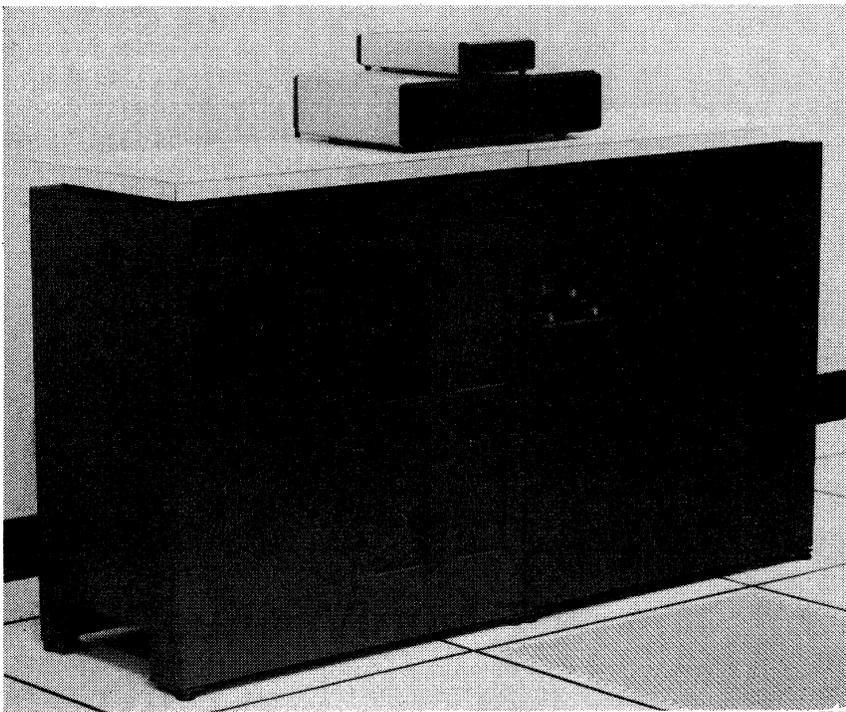
The Courier Virtual Terminal Line Controller (VTLC), is housed in the right cabinet. A cable-attached diskette controller and unit occupies the left cabinet. A Bell 4800 bps modem and line interface is pictured above the processor.
