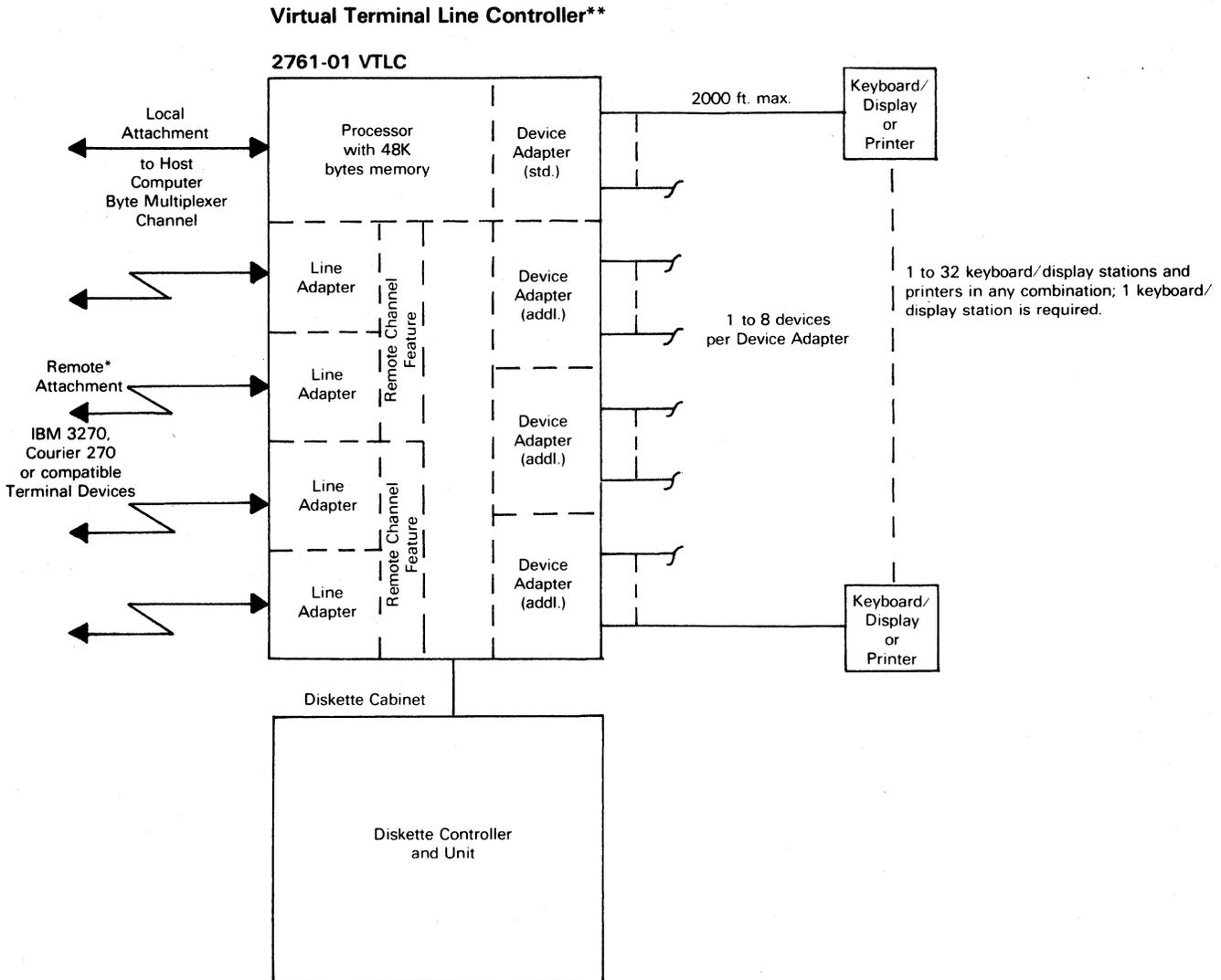
\*Each remote line may support up to 32 stand-alone terminals or cluster control units on leased, multipoint lines; total remote device capacity of 128 per VTLC system.
