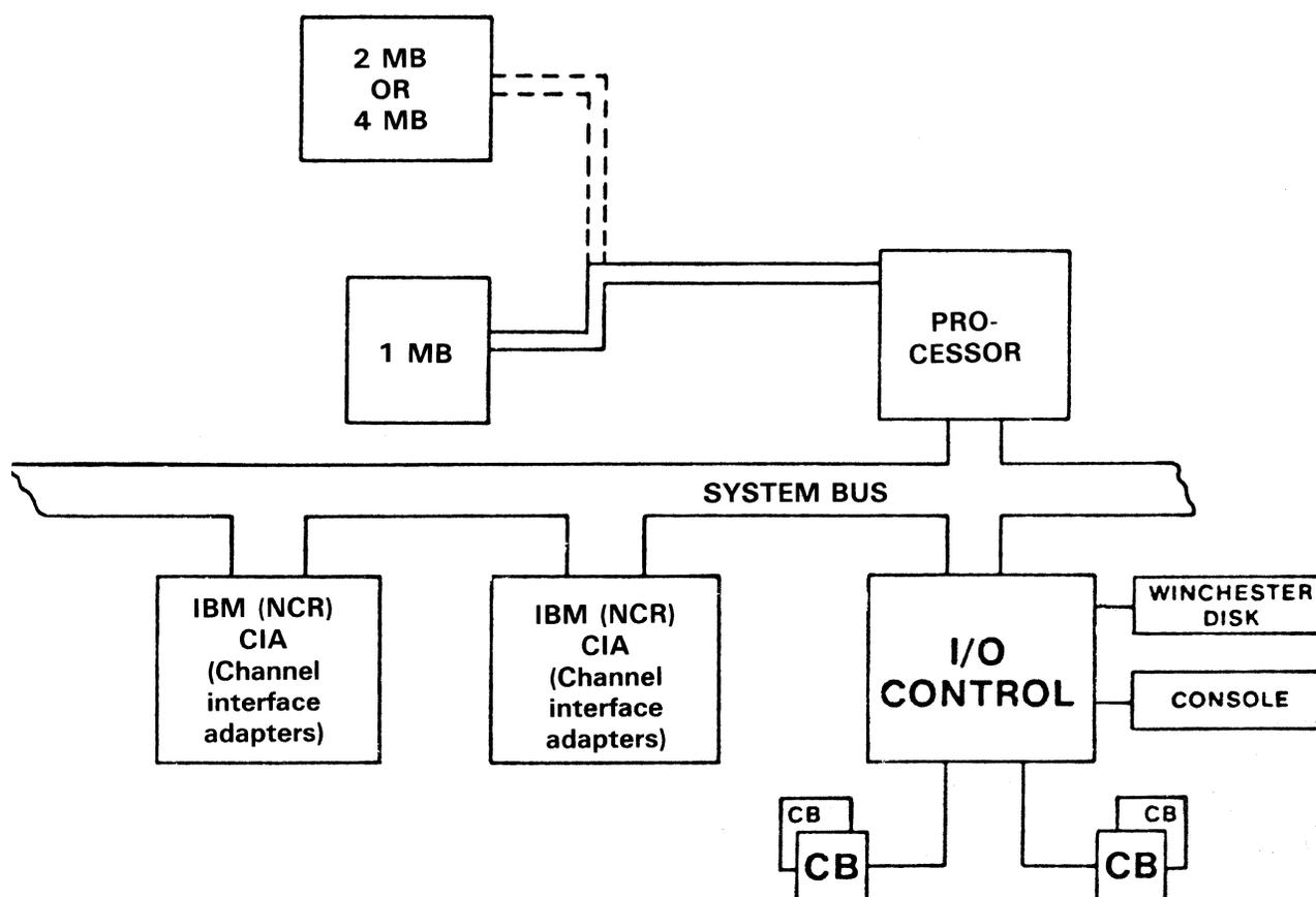
Figure 1. The basic Comten 5620 is made up of a central processing unit (CPU), a channel interface unit, a fixed disk drive, a communications subsystem, and an optional system console.
