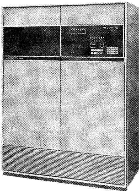
*NCR Comten's 3690 communications processor can be configured as a front end, standalone message switch, or remote communications processor. The 3690 models compete directly with IBM's 3725 processors.*
