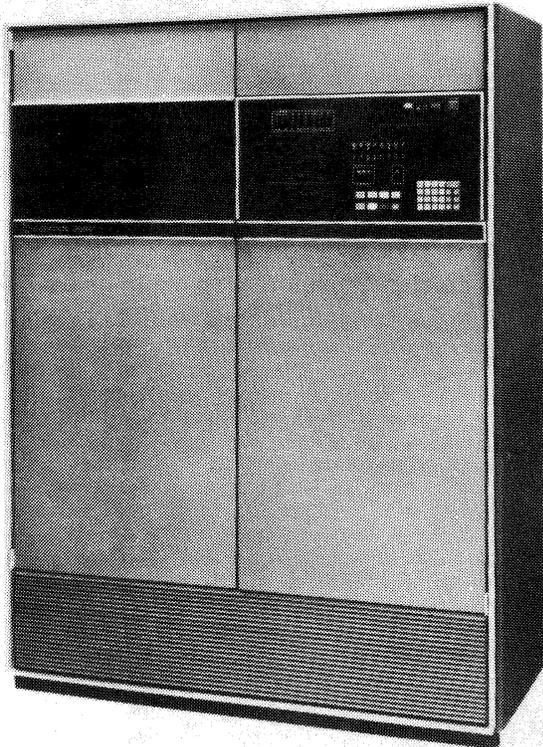
*The top of the line Comten 3690, shown above, is a worthy replacement of an IBM communications processor. It has up to four times the main memory capacity, supports more hosts simultaneously, and supports one and a half times as many communications lines.*
