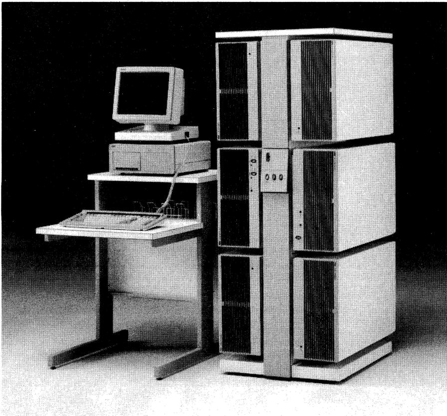
*NCR Comten's 5620XP communications processor is 2.2 to 3.7 times more powerful than the earlier Comten 5620, depending on software configuration. It supports up to 64 communications lines using asynchronous, bisynchronous, SDLC, or X.25 protocols. The Comten 5620XP can be used in both SNA and non-SNA network configurations.*
