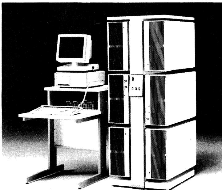
*NCR Comten's 5620XP communications processor supports up to 64 communications lines using asynchronous, bisynchronous, SDLC, or X.25 protocols. The Comten 5620XP can be used in both SNA and non-SNA network configurations.*
