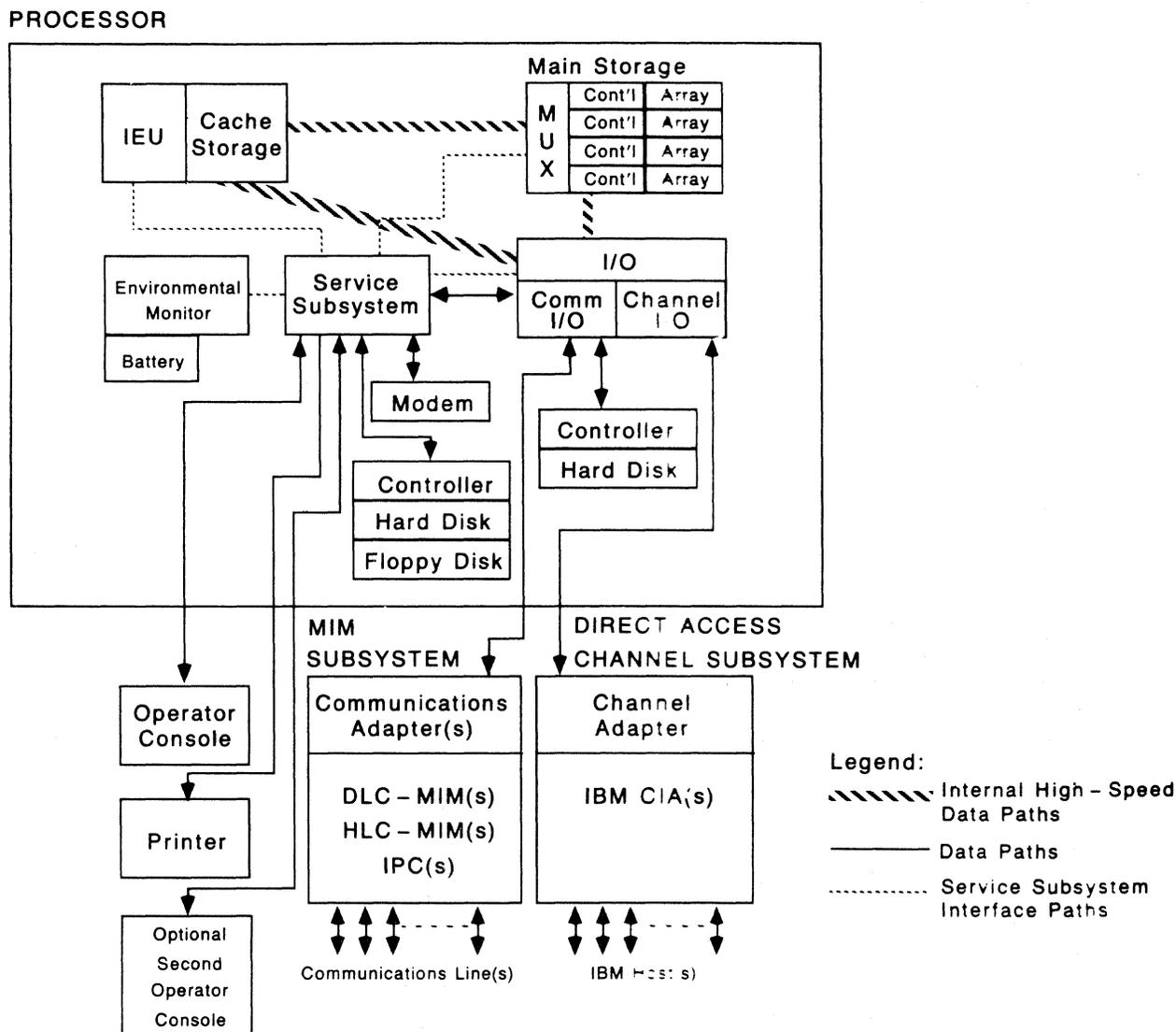
Figure 1. A block diagram of the Comten 5660 Communications Processor.
