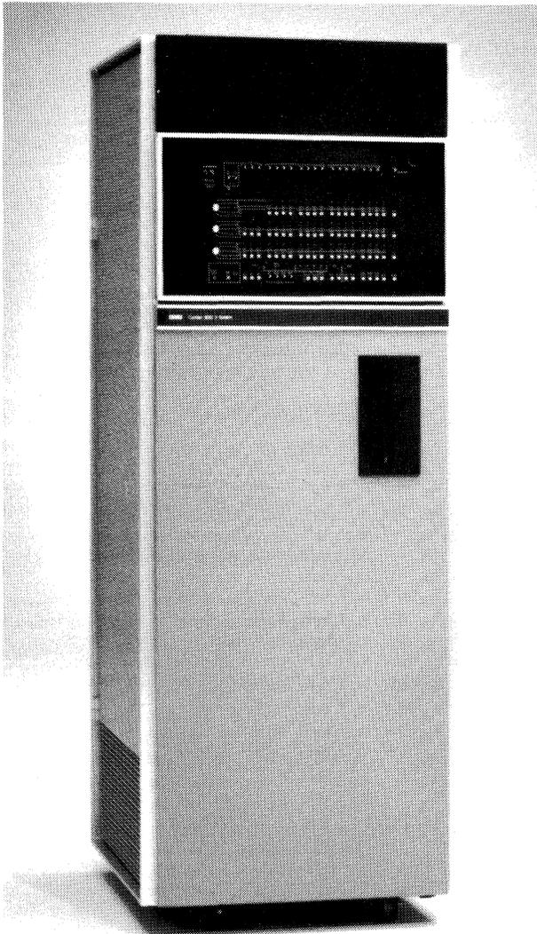
*NCR Comten's 3650 is available in 10 models. These models are the entry-level series of front-end and remote communications processors.*
