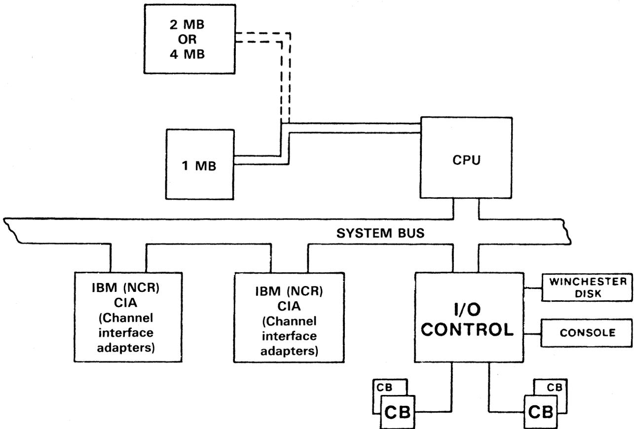
Figure 1. The basic Comten 5620XP is made up of a central processing unit (CPU), a channel interface unit, a fixed disk drive, a communications subsystem, and an optional system console.
