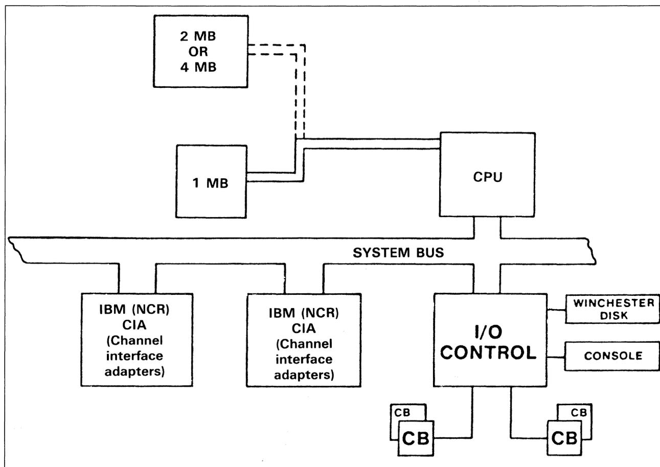
Figure 1. The basic Comten 5620XP consists of a central processing unit (CPU), a channel interface unit, a fixed disk drive, a communications subsystem, and an optional system console.
