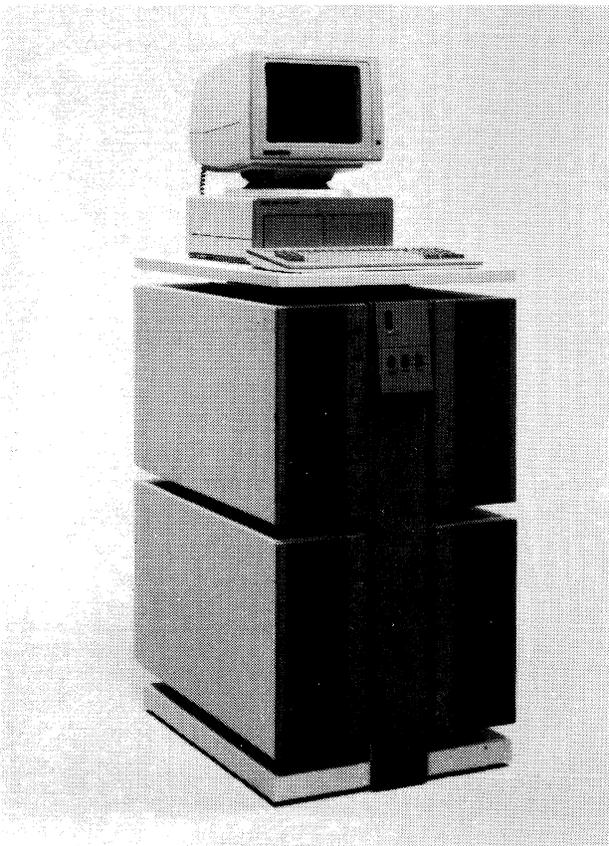
*NCR Comten's 5620 Communications Processor is the first member of the company's new generation of communications processors. The 5620 provides the same capabilities as Comten's larger models, the 3650 and the 3690.*
