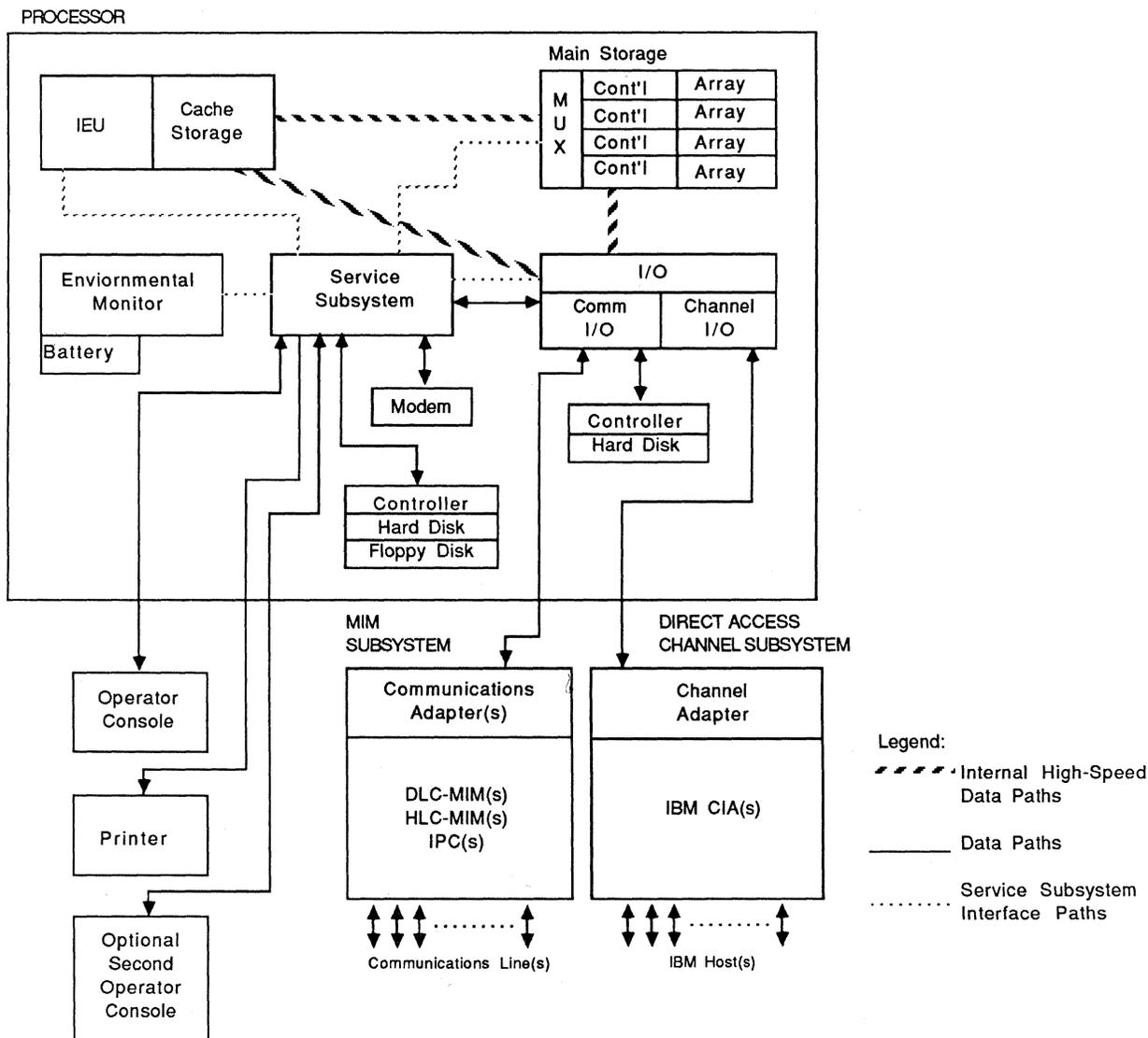
Figure 1. A block diagram of the Comten 5660 Communications Processor.
