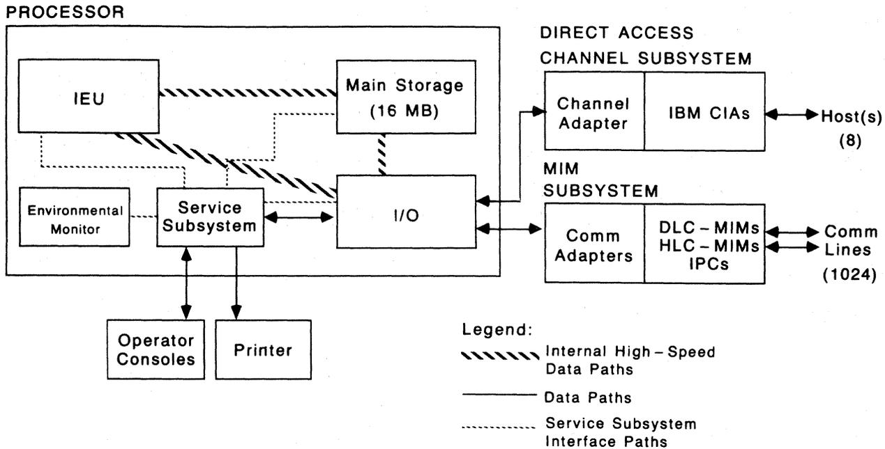
Figure 2. The Comten 5660 configured as a Front-End Processor.
