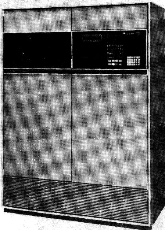
*The top of the line Comten 3690, shown above, is a worthy replacement of an IBM communications processor. It has up to four times the main memory capacity, supports more hosts simultaneously, and supports one and a half times as many communications lines.*
