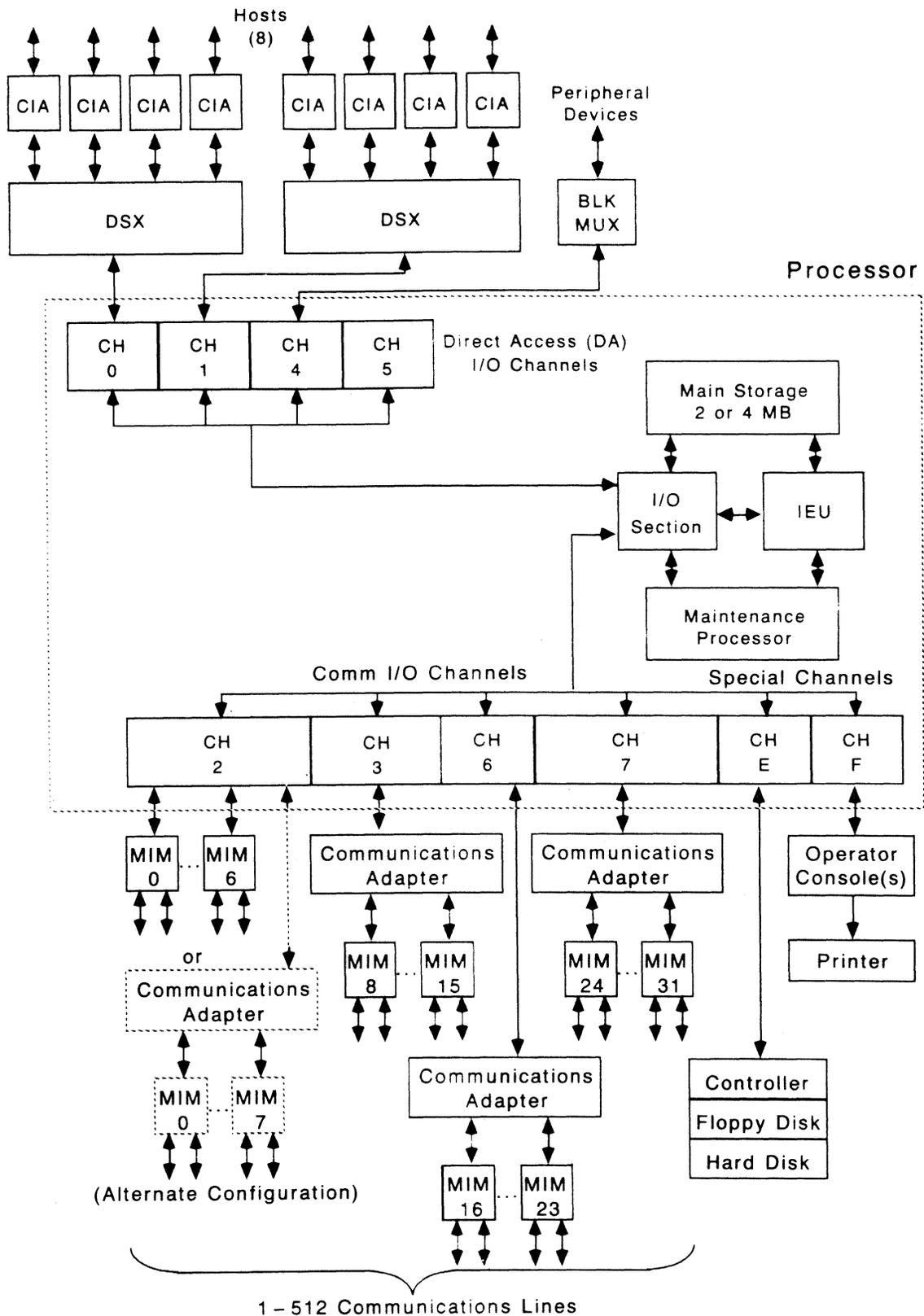
Figure 1. The Comten 3695 Communications Block Diagram.
