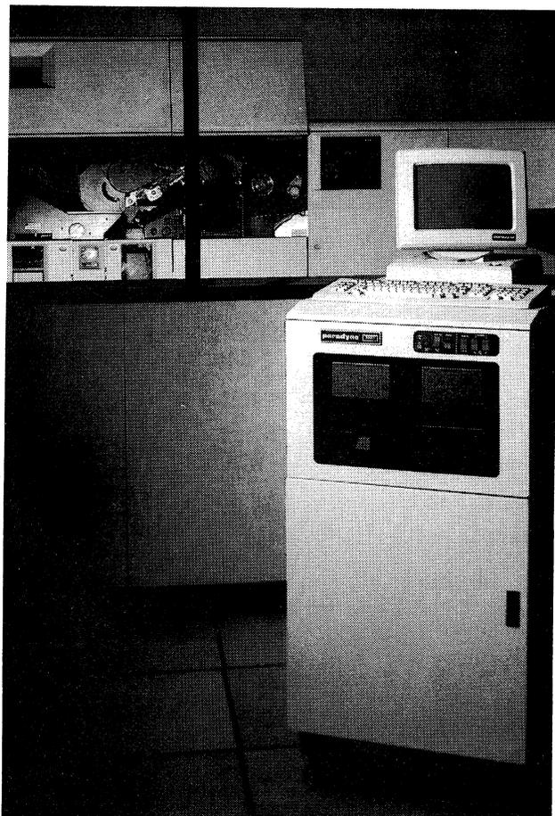
*Paradyne's PIXNET/XL system can simultaneously attach to two separate hosts and support 512 terminals.*
