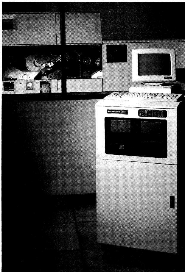
*Paradyne's PIXNET/XL allows remote peripherals to function as if they were in the same room with the host. This system supports up to 384 terminals.*
