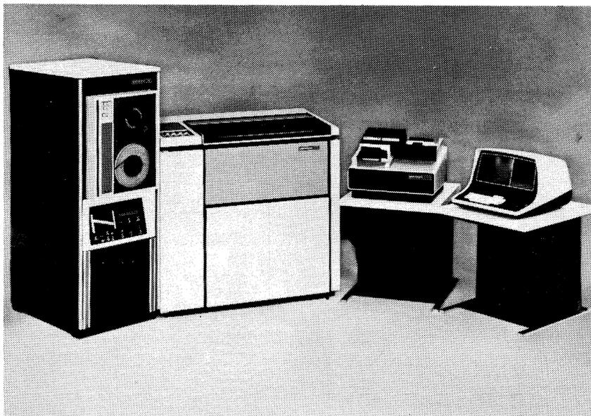
The PIX-II Remote Control Unit (RCU) is shown to the left with companion peripherals. The tape drive, line printer, card reader, and CRT peripherals, as well as high-speed synchronous modems can be furnished by Paradyne as part of the PIX system. PIX provides a virtual data link that causes the peripherals to react as if they were directly connected to the host computer even though they may be located thousands of miles away.
