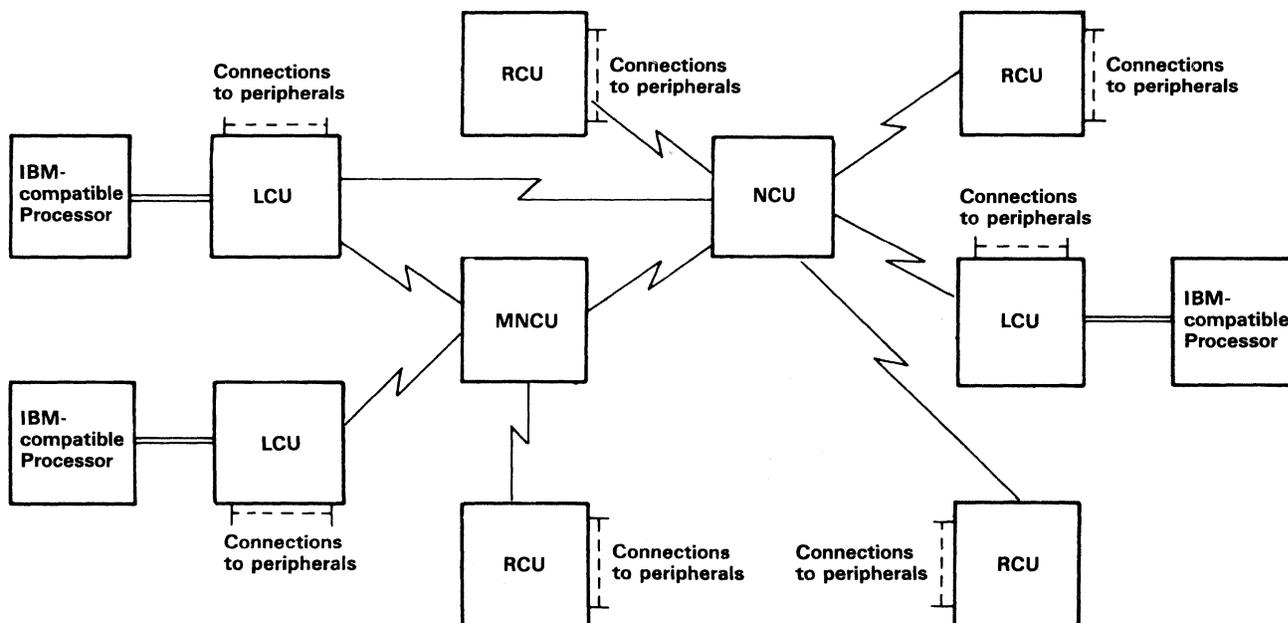
Maximum number of addressable devices per PIXNET system is limited only by line speed and throughput considerations.
