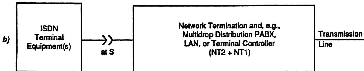
An implementation (see Figure 3c) where ISDN physical interfaces occur at reference point S but not T.
