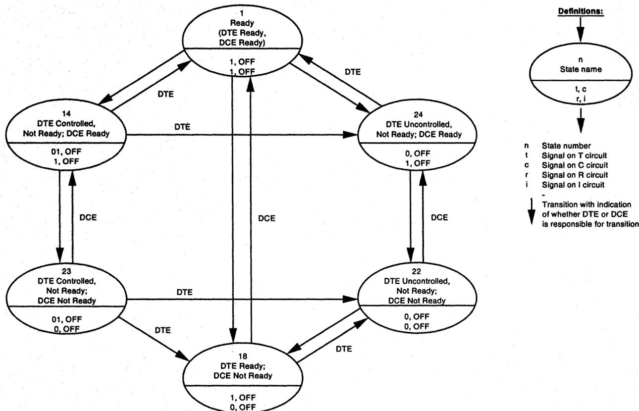
The above diagram indicates transitions that are allowed in X.21 networks. Other transitions are possible and may be allowed in some networks. See Table 3 for a listing of possible transitions.
