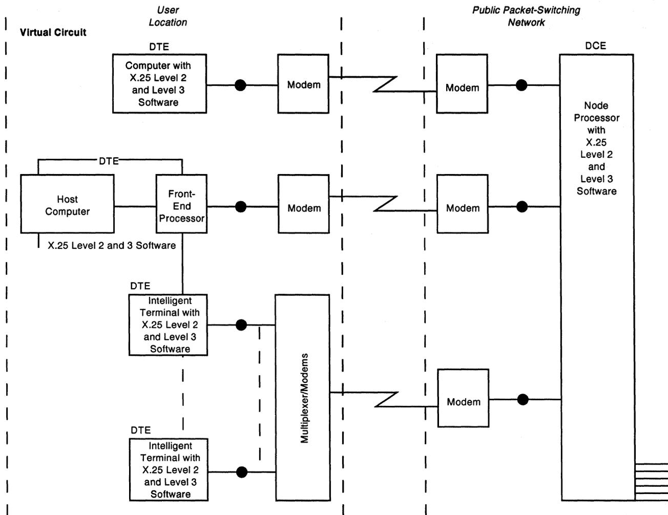
● Signifies an interface that must conform to X.25 Level 2, Physical Interface Standards.
