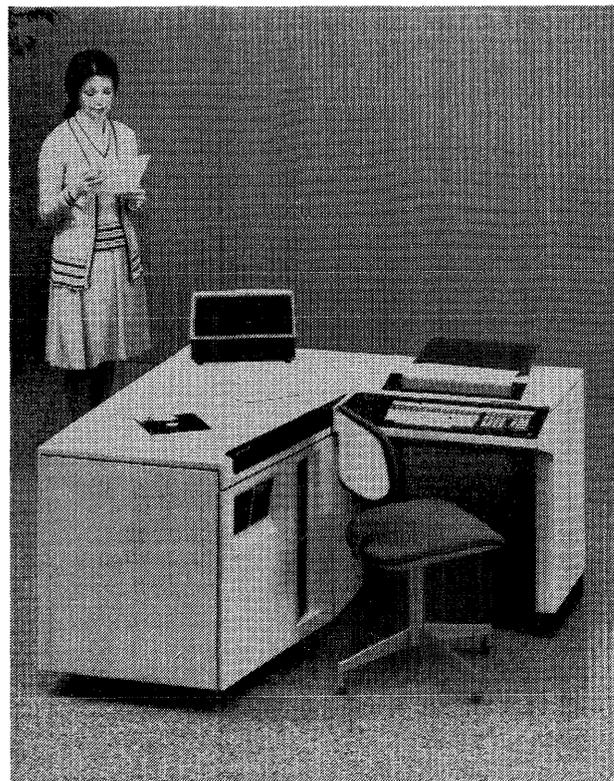
*The Burroughs B 80, an impressive new small business computer, doesn't look like a typical minicomputer. Its processor is hidden inside the cabinetry and is part of a neatly packaged system. The entry-level configuration includes 32K bytes of MOS memory, a 60-cps printer and keyboard, two floppy disk drives (1 megabyte each), a magnetic tape cassette drive, and a 256-character visual display terminal. It can be purchased for \$19,510.*
