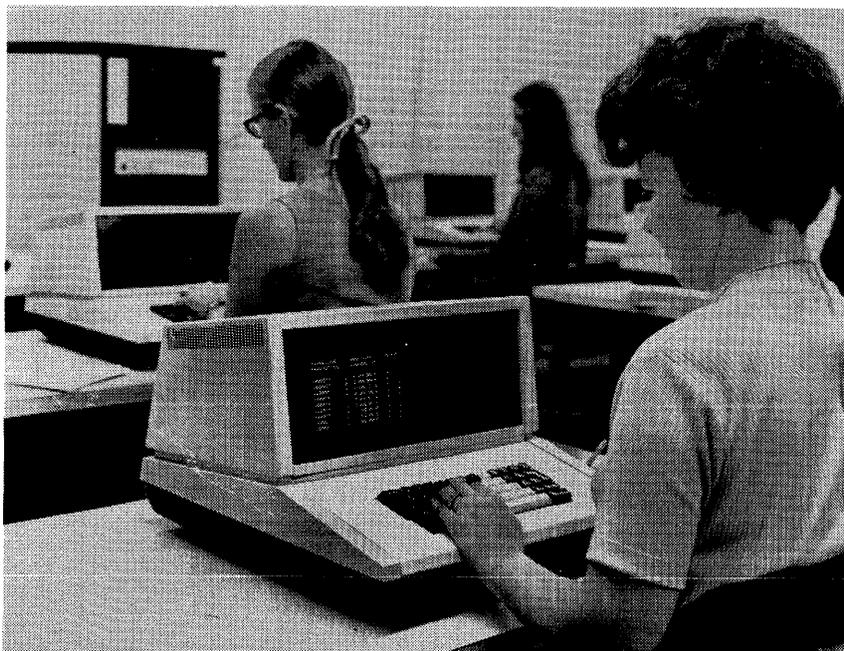
*The 1900 CADE System supports up to 32 of the CRT keystations shown here. The display is arranged in 12 lines of 40 characters each, and the keyboard is available in standard keypunch, keypunch/adding machine, or typewriter arrangements. The control processor cabinet is shown in the left background.*
