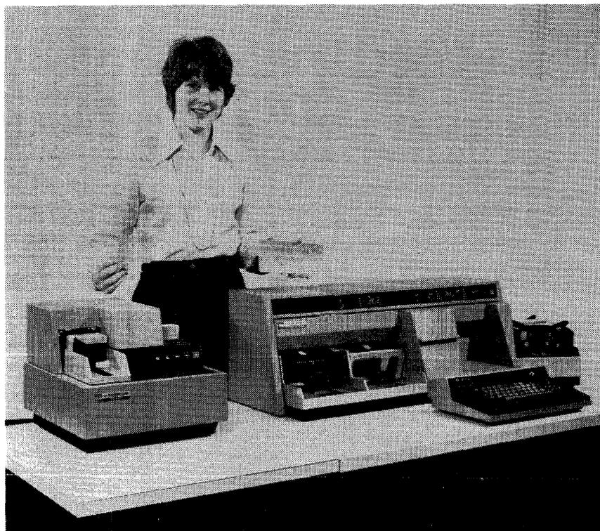
*This Decision Data 8010 Interpreting Data Recorder is shown with the optional 96-to-80-Column Card Converter (at left). The 8010's dual input hoppers can be seen at the far right, while the dual output stackers are clearly visible to the left of the keyboard.*
