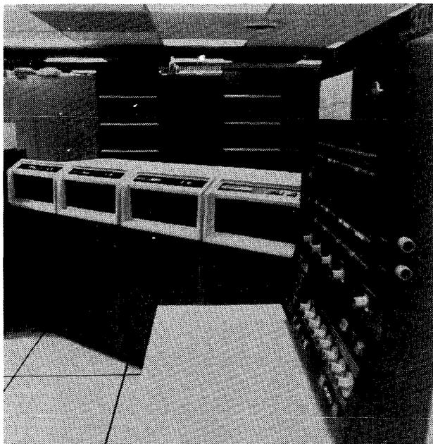
*The CDC 33801 Disk Subsystem provides up to 12.8 billion bytes of storage for users of IBM System/370 Model 145 and larger computers.*
