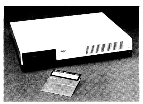
AT&T's 3B2/310 supports up to 14 simultaneous users and employs a WE 32100 processor. The 3B2/310 supports up to 4MB of RAM and a maximum of 432MB of hard disk storage.
