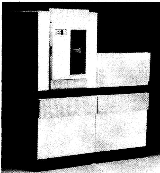
The 3B15, comprising Models 101, 201, and 301, is the new mid-range system in AT&T's 3B Computer family. The 3B15 supports up to 60 simultaneously active users. It runs under Release 2.1 of Unix System V, which provides demand paged memory management and record/file locking.
