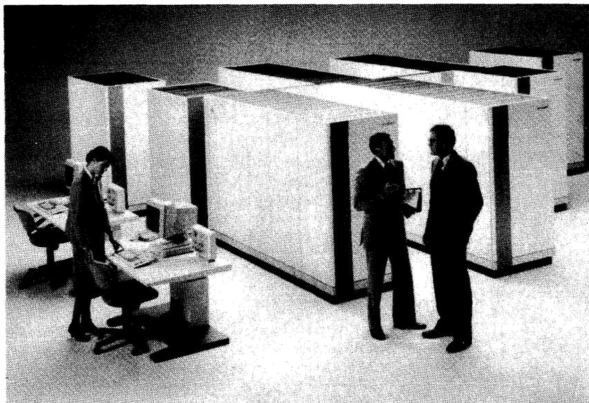
*Billed as the most powerful general-purpose mainframe ever built for the System/370-compatible marketplace, the Amdahl 5990 Model 1400 has a CPU cycle time of 10 nanoseconds and can process up to 115 million instructions per second, by industry estimates.*
