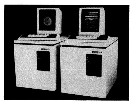
Apollo's Domain Systems, Models DN300, DN420, and DN600, are 32-bit VLSI systems that offer from 512KB to 3.5MB of main memory, up to 768 megabytes of disk storage, and the ability to support multiple concurrent processes, with each process having a virtual address space of up to 16 megabytes.
