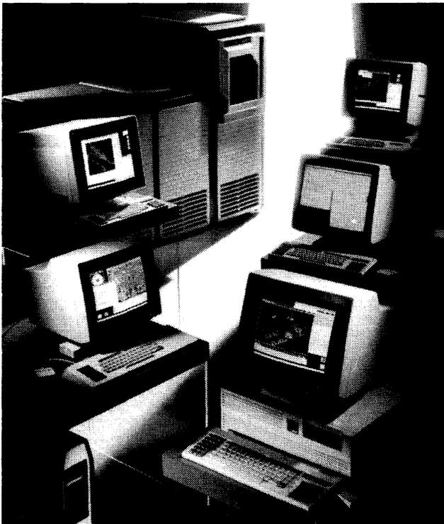
*Apollo's 32-bit Domain Systems supply a range of Unix-based computing resources for the technical workgroup environment. Left (bottom to top) DN570 with a 15-inch color monitor, high-end DN580; and top of the line DSP9000 compute server. Right (bottom to top) Series 3000 with a 15-inch color monitor; Series 3000 with a 19-inch monochrome monitor; and DN570 with a 19-inch color monitor.*
