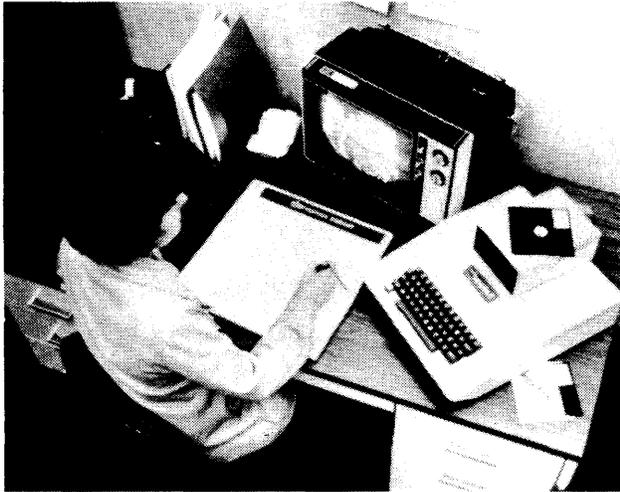
*The Apple II, configured for fairly typical home use, includes a single diskette drive and a TV set for color graphics. Not as commonly used is the graphics tablet shown here, capable of producing high-resolution, multi-colored drawings.*
