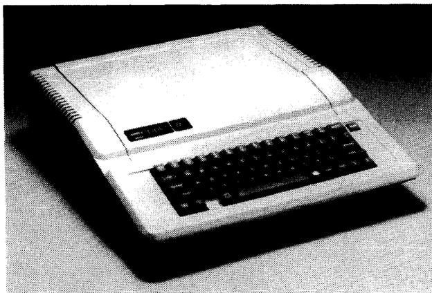
*The Apple IIe was designed as a replacement for the Apple II computer. It provides 64K bytes of RAM expandable to 128K, an upper and lower case alphabet, and an extensive array of software.*
