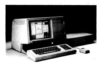
The Apple Lisa is a 32/16-bit personal computer featuring six integrated software packages covering office applications. Its standard configuration includes the CPU, 12-inch CRT display, detachable-keyboard, 1MB RAM, 1.7MB diskette storage capacity, 5MB hard disk storage capacity, and a mouse.
