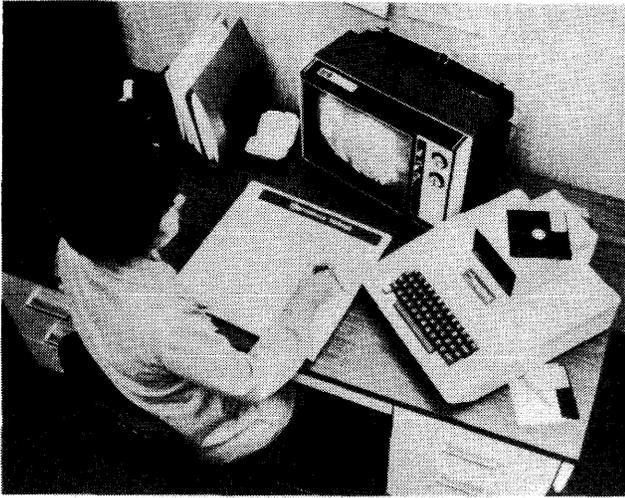
*The Apple II configured for fairly typical home use, with single diskette drive and TV set for color graphics monitor. Not as commonly used is the graphics tablet shown here, capable of producing high-resolution, multi-colored drawings.*
