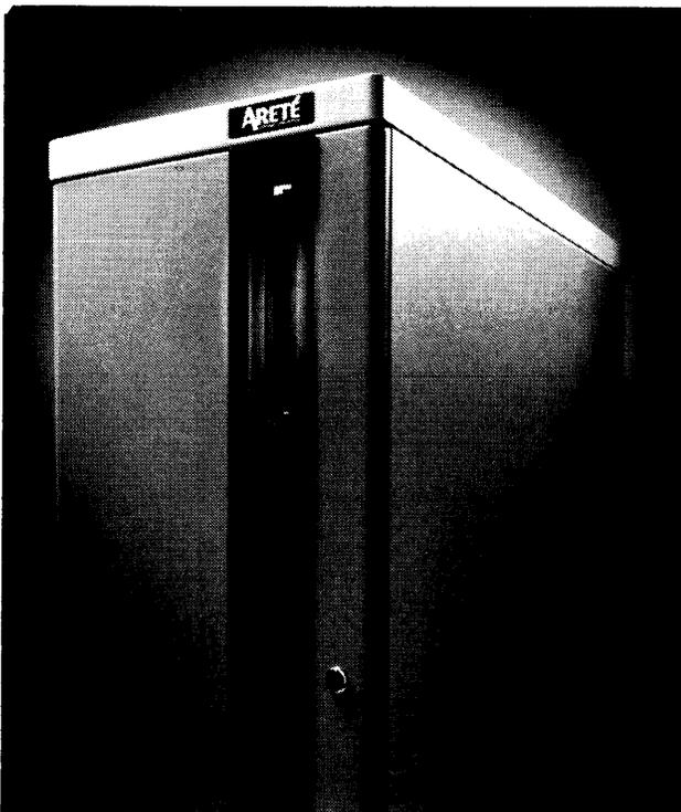
*The Arété Series 1000 comprises three models which support from 2MB to 16MB of main memory and from 168MB to 8GB of disk storage. Up to 256 users are supported on the Unix-based supermicro system.*
