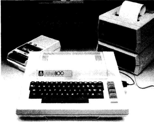
The Atari 800 shown here consists of a 16KB RAM, a cassette program recorder, a 40-cps 4-inch roll printer, a 5 1/4-inch 92KB mini-diskette drive, and a user-supplied color TV set or monitor. Total cost of this system is about \$2,200. Programs can be loaded either via plug-in ROM cartridges, cassette tapes, or diskettes. The 800 is programmable in BASIC or Assembly language.
