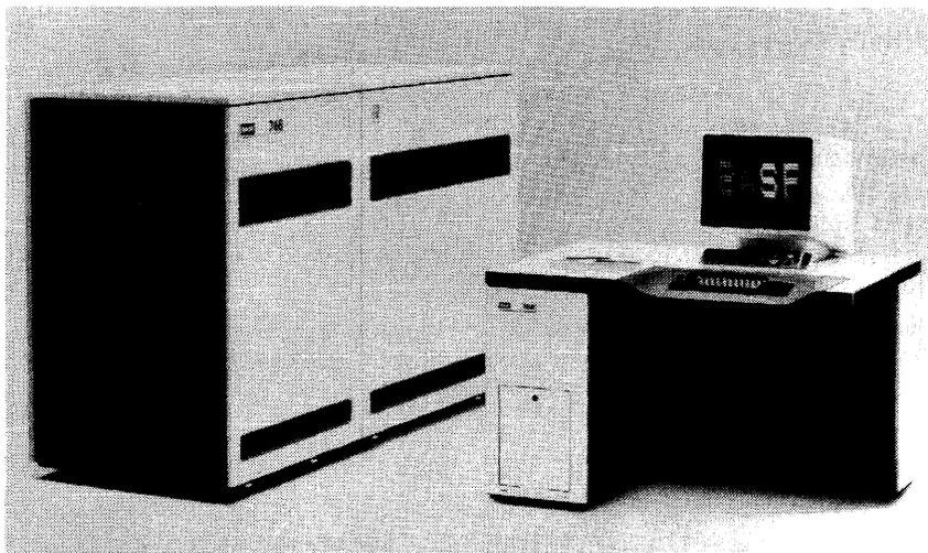
*The BASF 7/68, a plug-compatible substitute for the IBM 4341-2, is based on the Hitachi M240H and can support both IBM and BASF peripherals. BASF reports that tests show that the 7/68 operates about twice as fast as the 4341-2 while taking up less space and generating less heat.*
