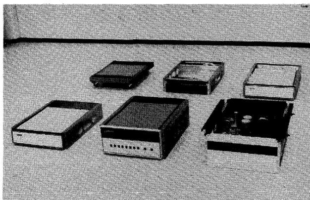
Here are two exploded views of a BTI 4000 Series system showing the company's unique stack-mounting technique. The individual chassis (at left) form the cabinet, and the skins (side panels) simply lock onto the stacked chassis, binding the stack into a rigid structure. Index pins on the upper side of each chassis mate with holes on the lower side of the next one, providing a flexible mounting system. Individual units can be removed from the special shells for service.
