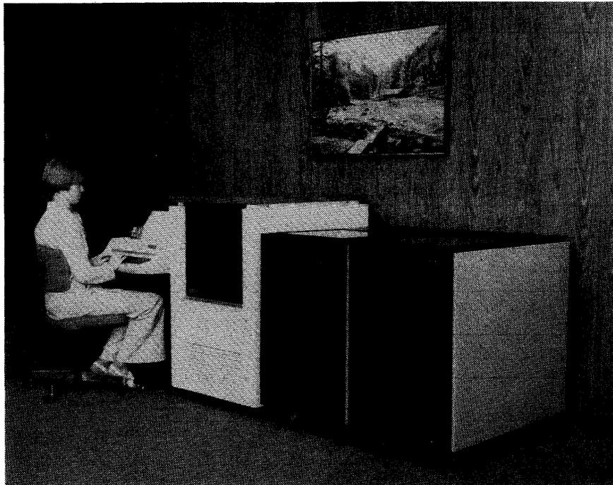
▷ memory, eight user ports, and one 2.4-megabyte cartridge disk drive. Port capacity could be increased to 16 ports. Storage could be expanded by adding up to three 2.4-megabyte drives to the disk controller in the basic system, and the storage capacity could be further extended by adding more disk controllers as required.
