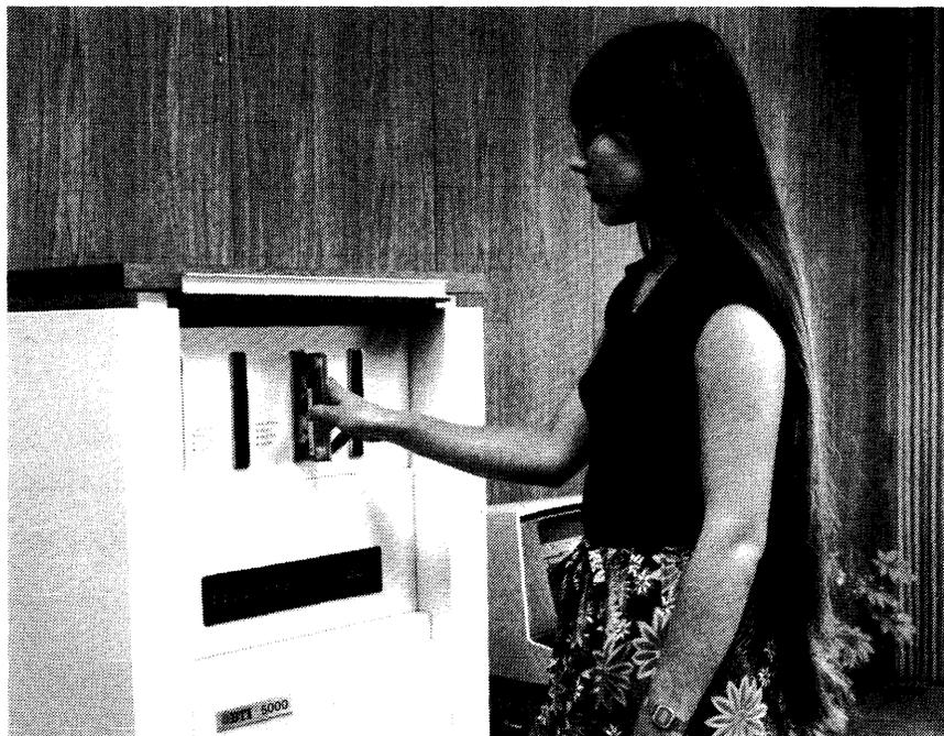
This photo shows the BTI 5000 system cabinet with the plexiglass cover lifted. The magnetic tape cartridge module (with four drives in this version) and the CPU are below this unit. The disk drives and system power supply are behind the cover panel, below the CPU.
