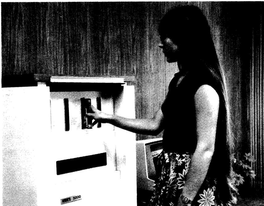
The basic BTI 5000 system includes a magnetic tape cartridge drive for software backup and recovery. With four drives installed, up to 40 megabytes can be transferred without physical handling of the tape cartridges.
