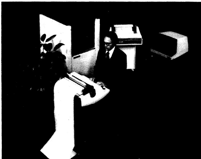
The BTI 5000 is shown here with the optional Model 5620 (300 lpm) line printer to the right of the processor cabinet. Terminals utilized by the BTI 5000 include Hazeltine CRTs or Texas Instruments' Model 1800 teleprinters.
