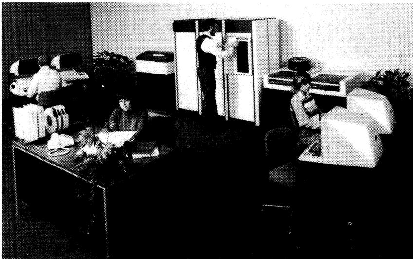
The BTI 8000 supports a number of peripheral devices and terminals. The BTI 8000 configuration shown here includes four terminals, two disk-pack drives, a reel-to-reel magnetic tape unit, and a line printer. This 32-bit system can support up to 200 interactive users in a multilanguage, multifunction environment.
