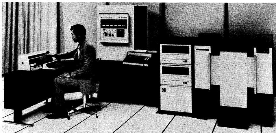
*This basic B 1700 configuration consists of (from left): 96-column card reader/punch equipped for off-line use as a data recorder, central processor with console printer, dual disk cartridge drive, and line printer.*
