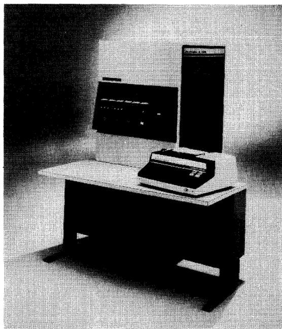
*This B 1705 basic system, the smallest B 1710-based system, is offered to users who wish to configure their own systems rather than choose one of the packaged B 1700's. The system includes a CPU with 24K bytes of main memory and a 160-lpm console printer/keyboard.*
