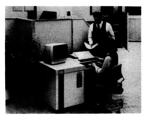
The B 92 is available with up to 512K bytes of main memory and 11 I/O channels, 4 of which may be communications channels. Peripherals available include several types of diskette drives, 2 different fixed disk drives, 2 different cartridge disk drives, 2 magnetic tape cassette devices, 9 line printers, and a variety of terminals. The B 91 and B 92 are capable of running under CMS or ACSYS software.
