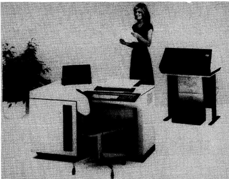
*The entry-level B 80-20 system is available with a variety of disk configurations: up to two BSM diskette drives, a cartridge disk subsystem with a total capacity of up to 18.4 megabytes, a combination BSM drive and fixed-disk subsystem with a total capacity of 19.8 megabytes, or a combination of cartridge disk and fixed disk with a total capacity of 28 megabytes. Purchase price for the basic B 80-20 system with two BSM drives is \$17,065.*
