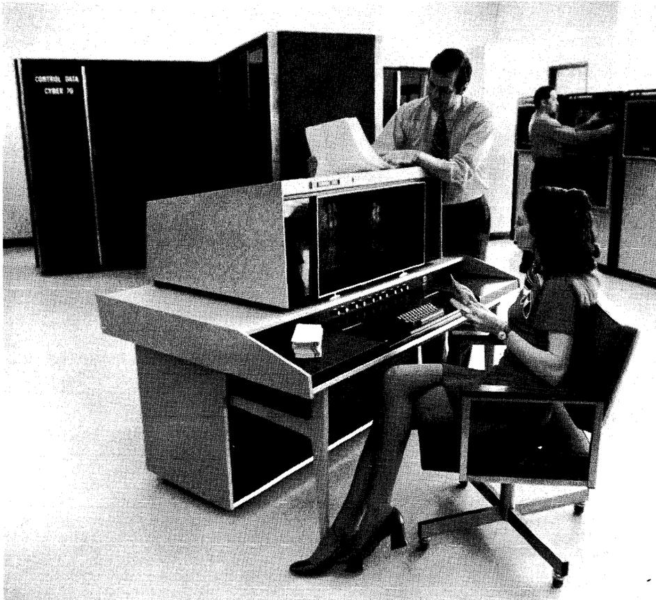
*The Cyber 70 System Console features dual CRT displays and a typewriter-style data entry keyboard.*
