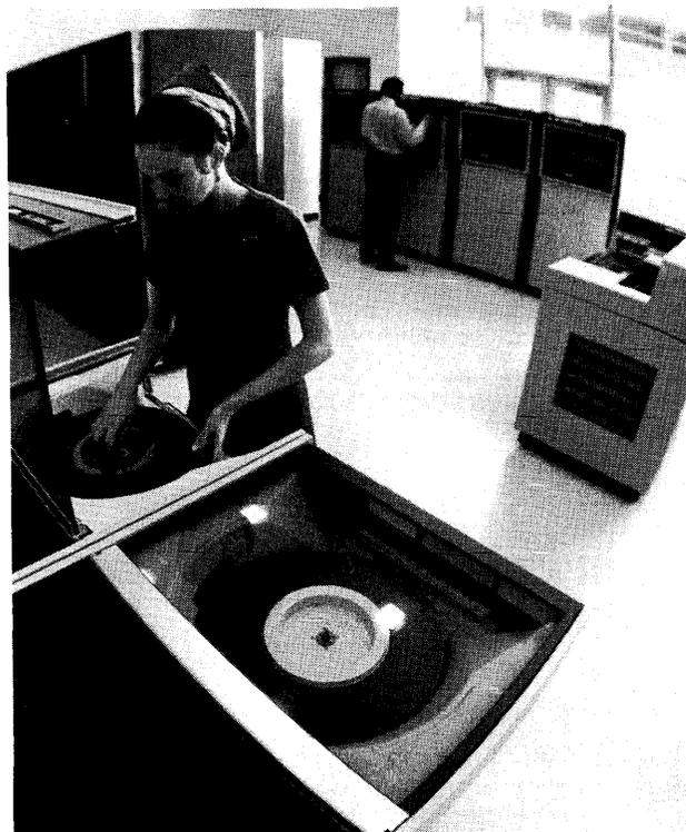
*Control Data's new 844-2 Disk Storage Units store up to 118 million characters per spindle, transfer data at 1.13 million characters per second, and have an average head movement time of 30 milliseconds.*
