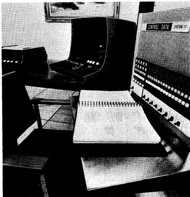
*The general-purpose CDC System 17 Series offers 4K to 64K 16-bit words of either 600-nanosecond or 900-nanosecond MOS memory, a wide range of CDC-built peripherals, three levels of operating system support, and dozens of major application programs. Shown here is the System 17 CPU with a CRT operator console.*
