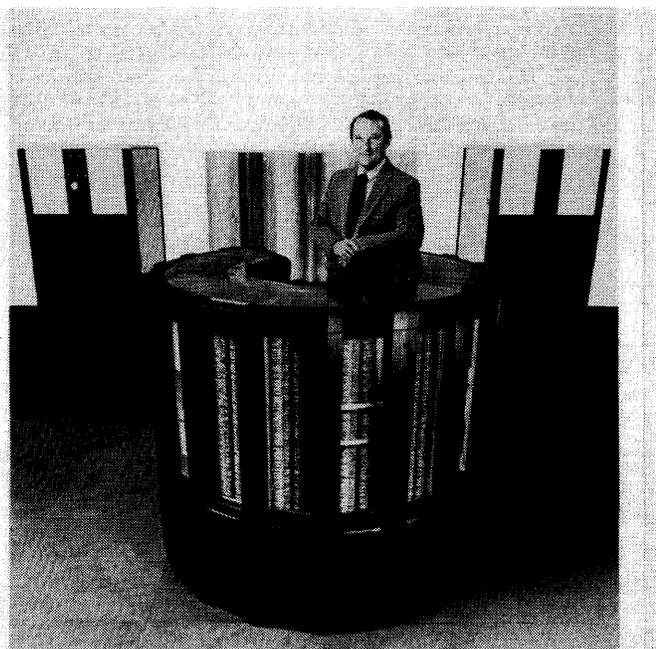
*The Cray-2 is the fastest computer system currently available. The system includes four 4.1-nanosecond central processors and 2 gigabytes of main memory. One compact circular unit houses the memory, computer logic, and DC power supplies. The Cray-2 occupies only 16 square feet of floor space.*
