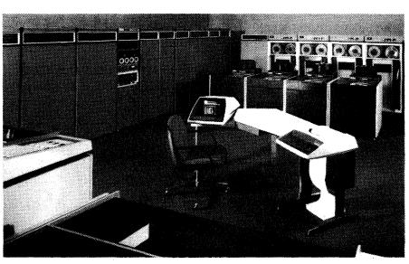
that provide double-precision addition, subtraction, division, and multiplication of fixed-point operands and a string manipulation instruction that performs decimal/binary conversions and editing functions. The cache has a 160-nanosecond access time, which, according to DEC, allows an effective memory cycle time of 334 nanoseconds.
