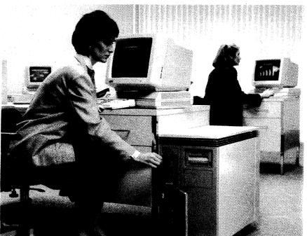
Digital Equipment Corporation's MicroVAX II delivers between 70 and 110 percent of the performance of a VAX-11/780 supermini. It is based on Digital's proprietary MicroVAX 78032, a full 32-bit microprocessor. Available in a variety of packaged configurations and building blocks, the MicroVAX II can accommodate up to 9MB of main memory, 1.8GB of Winchester disk storage, and 33 workstations.
