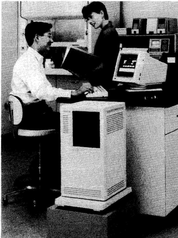
*Digital Equipment Corporation's newest MicroVAX systems, 3300 (pictured above) and 3400, support dual-ported strings of Digital's new RF30 Winchester storage unit; this scheme supports Digital's push into distributed transaction processing. Specialized laboratory data collection and workstation server configurations are also available.*
