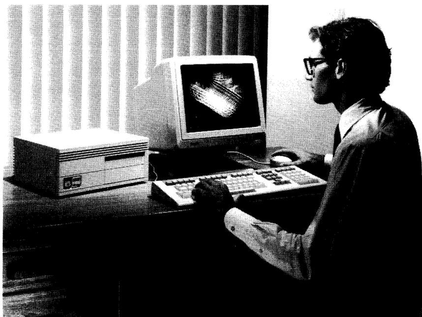
*Digital Equipment Corporation's VAXstation 2000 is available with 15- and 19-inch monochrome and color monitors. This desktop technical workstation is designed for use in networked and clustered configurations and is suitable for both technical and commercial computing in corporate environments. The workstation runs Digital's proprietary MicroVMS operating system and VMS Workstation Software or the Ultrix-32m operating system and Ultrix-32w workstation software.*
